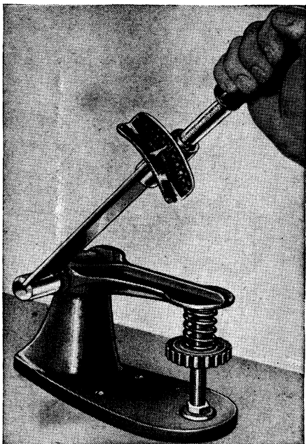
Fig. 17 Fixture and torque wrench for checking valve spring tension
