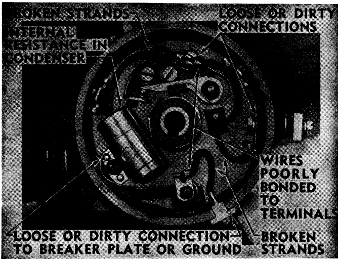
Fig. 1 Points of resistance in condenser circuit
