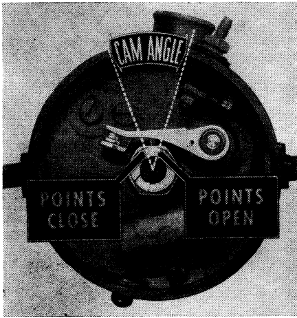
Fig. 25 Cam angle or dwell is the number of degrees of breaker cam rotation from the time the points close until they open again
