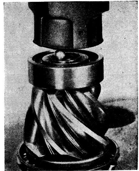
Fig. 50 Method of staking pinion shaft, using a bearing ball under a press ram
