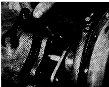
Fig. 44 Add or remove shims from pack under sleeve to obtain correct adjustment of shift fork pads in shift collar
