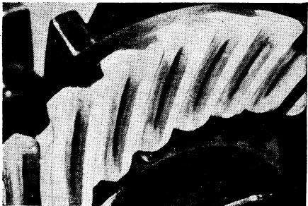
Fig. 39 Low narrow contact. To correct, move pinion away from bevel gear
