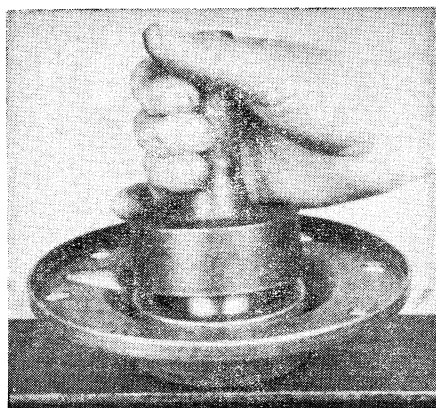
Fig. 84 Using seal driver to install pinion shaft oil seal
