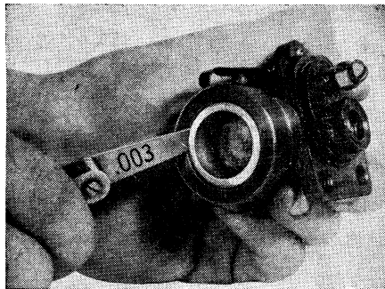
Fig. 17 Checking wheel cylinder piston fit with feeler gauge
