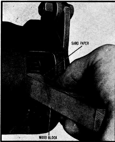
Fig. 14 Cleaning commutator with strip of sandpaper (00) placed over a wooden block
