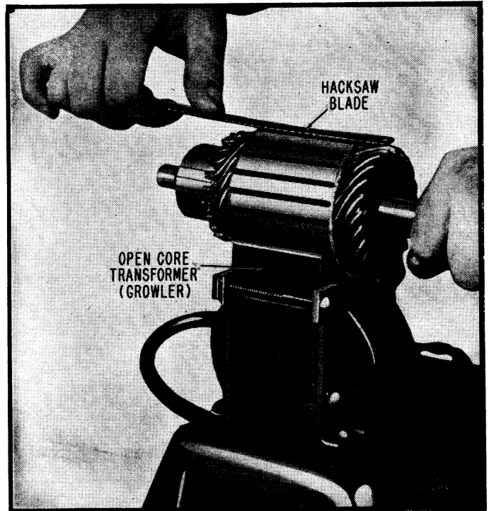
Fig. 13 Checking armature for short circuit with a growler. As armature is rotated by hand, steel strip (hacksaw blade) will vibrate if short circuit exists
