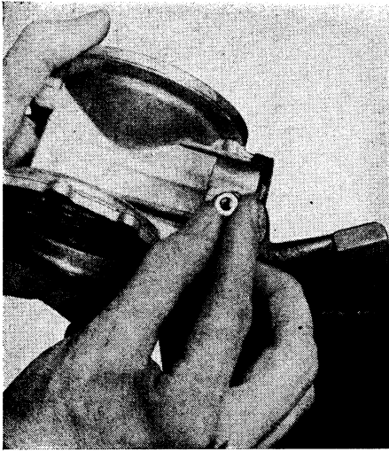
Fig. 38. Series AJ. Installing washer over small end of rocker arm pin. Turn washer until it lies flat
