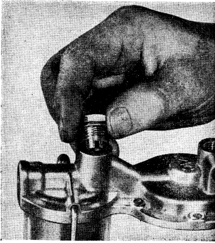
Fig. 17 Series B. Installing inlet valve chamber plug
