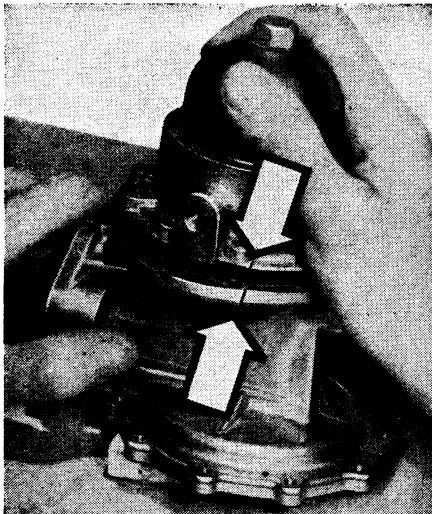
Fig. 39 Series AJ. Assembling body to cover, matching marks previously made
