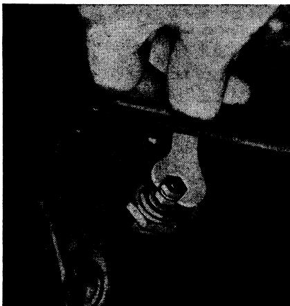
Fig. 12 Disconnecting wire from electric type temperature gauge
