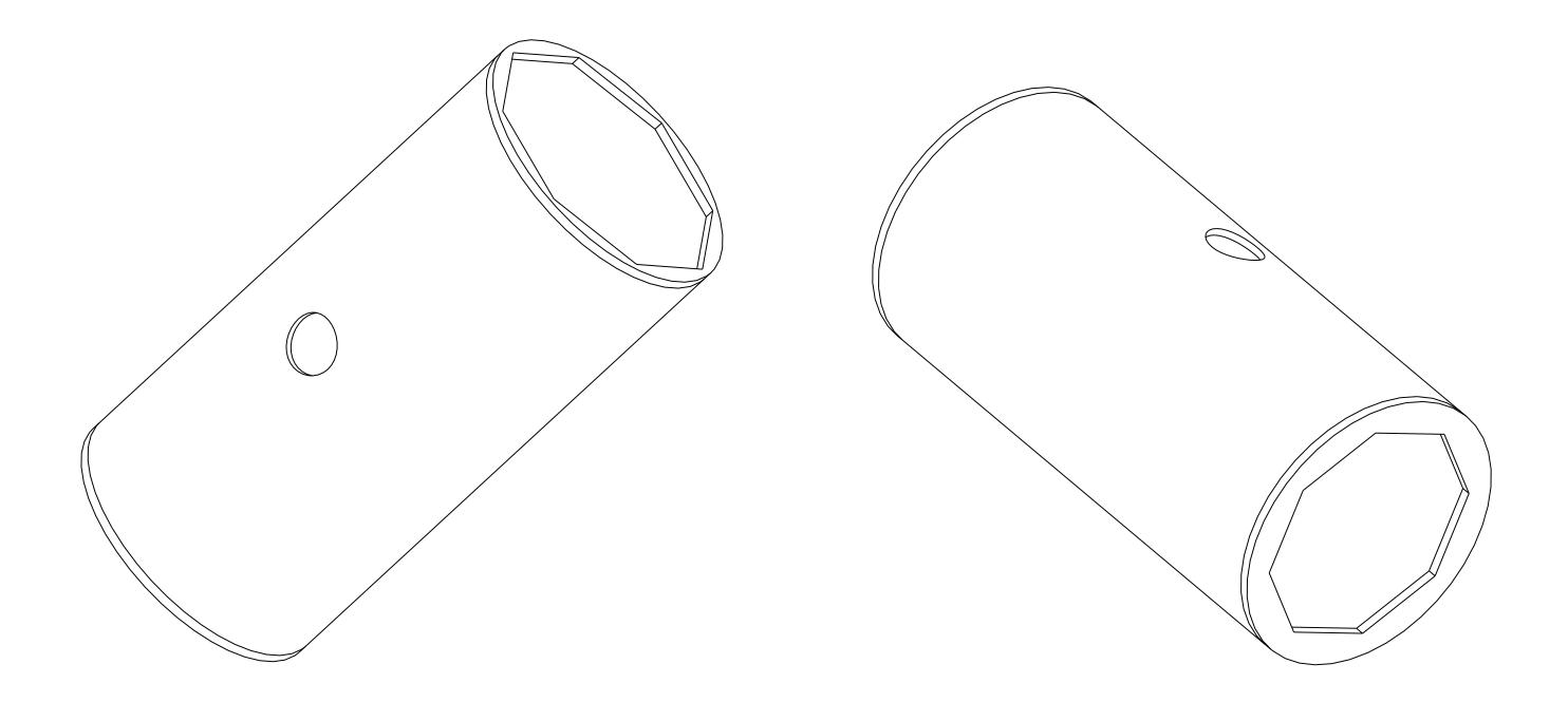
NOTES: 1. WELD HEX PLATE CUTOUTS TO 3" O.D. STEEL WALL TUBING 2. DRILL .625 THRU TUBE FOR HANDLE
