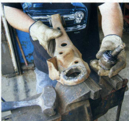
20 Once the ball joints were removed from the lower control arms, the control arms were completely bead-blasted and prepped for the installation of new ball joints and spray-painted black.
