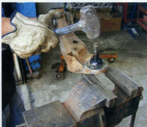
19 Using the same procedure as above, Bob used a powerful direct blow with the two-pound hammer to knock the lower control arm ball joints out.
