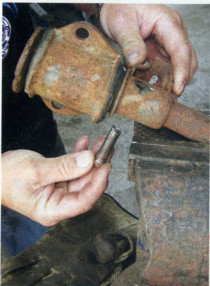
25 With the pin driven out, the torsion bar end was twisted off.
