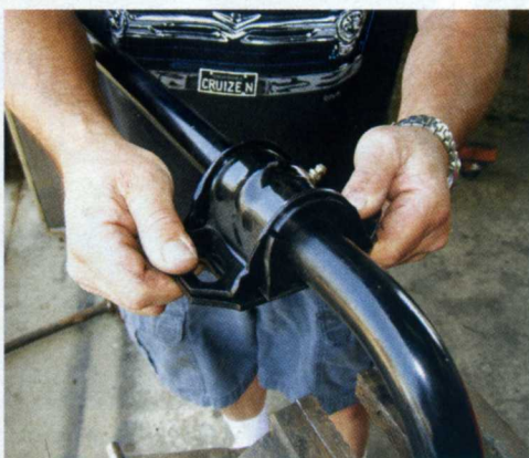
16 Then the zerk fitting was screwed into the new Bob's clamshell half and installed.
