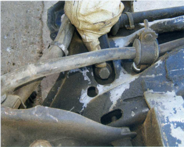
2 The first step Bob took to disassemble the Volare frontend was to back the tension off (unload) of the torsion bars.
