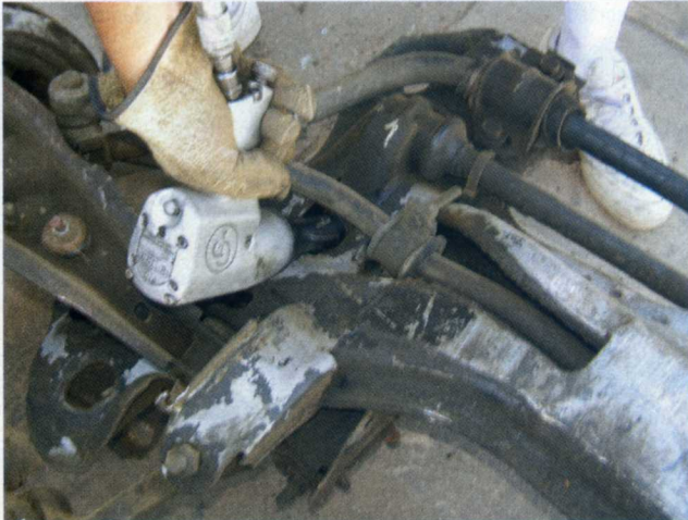
3 It can be done by hand with a ratchet or a breaker bar in a counter-clockwise direction (righthand threads), but Bob used an air impact wrench to make short work of it.
