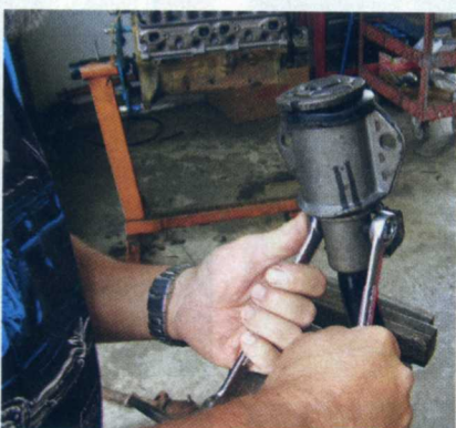
28 Bob used a Nylock nut to cap the 3/8-inch bolt, making sure the bolt was not over-tightened, which would cause the new torsion bar end to distort.
