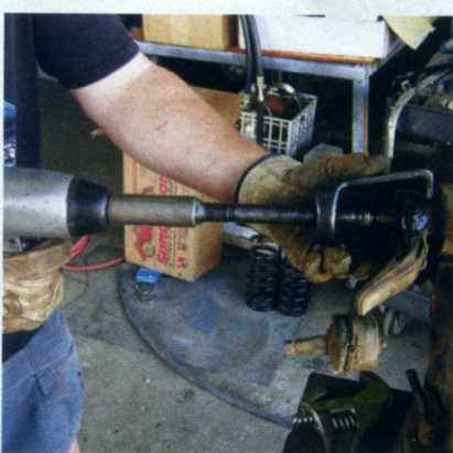
30 If the Pitman arm is stubborn, a Pitman arm puller will be necessary—the job will go a lot easier with one.
