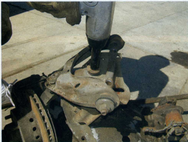
4 Ditto for removing the shock absorbers, which are not included in Bob's Volare suspension rebuild kit, but unless yours are nearly new, they should be replaced.
