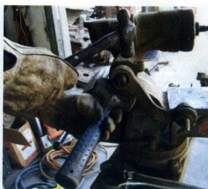
29 Bob demonstrated the Pitman arm could be removed without a Pitman arm puller by banging on one side of the arm with a hammer and backing up the other side with a hammer.
