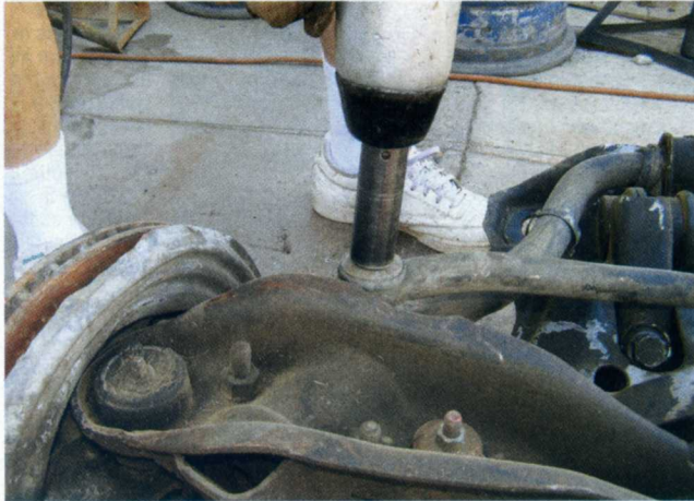
5 Next, the stabilizer bolts and stabilizer hardware at the stabilizer bar ends, including the rubber donuts, were removed. Bob's kit includes all the stabilizer bar hardware that should be replaced, including new rubber donuts.
