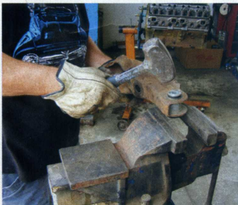
17 A two-pound hammer with a socket used as a drift knocked out the lower control arm bushings.
