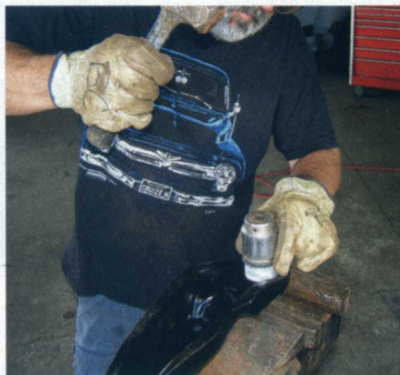
21 Bob securely positioned the lower control arm on the vise and used a large (whatever size will fit snugly over the ball joint) socket driven with a two-pound hammer to install the ball joint into the lower control arm.
