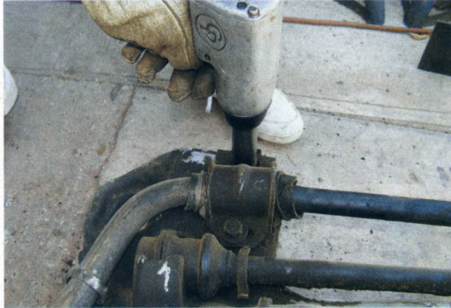
6 Forward of the stabilizer ends are the "clamshells" that attach the stabilizer bar. From the factory these were not replaceable individually, and the complete stabilizer bar assembly is now obsolete. Bob's rebuild kit includes nylon liners that replace the formerly unserviceable part with an upgraded design.
