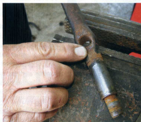
23 Part of doing a thorough rebuild job includes an inspection of the upper control arm cross-shaft to ensure the serrations aren't excessively worn.
