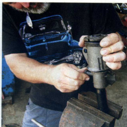
27 The original pin was discarded and a new Grade 8 3/8-inch bolt was pushed into place.
