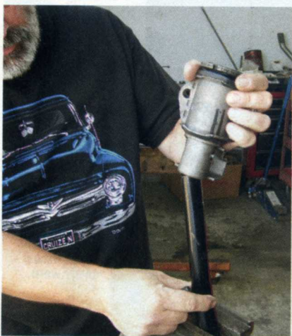
26 The new replacement part from Bob's F-100 Parts was twisted on in the same manner as the old part twisted off.
