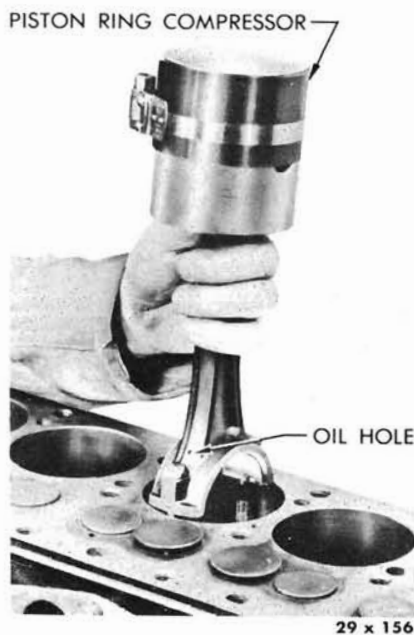
Figure 25—Installing Piston and Connecting Rod Assembly with Tool C-385
