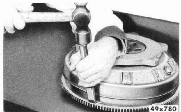
Figure 53—Driving Ring Gear Off
