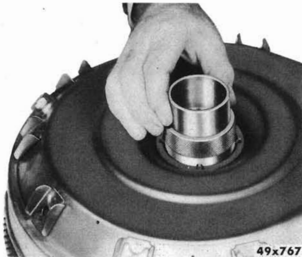
Figure 68—Pushing Seal Ring Off Locators Using Pilot (Tool SP-788, Part of Tool C-885)
