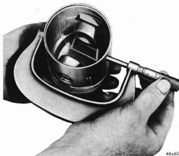
Figure 27—Measuring Piston with Micrometer Calipers
