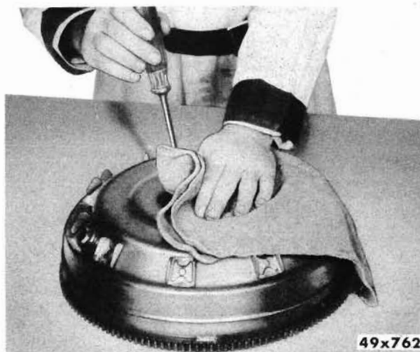
Figure 63—Method of Retaining Snap Ring and Spring
