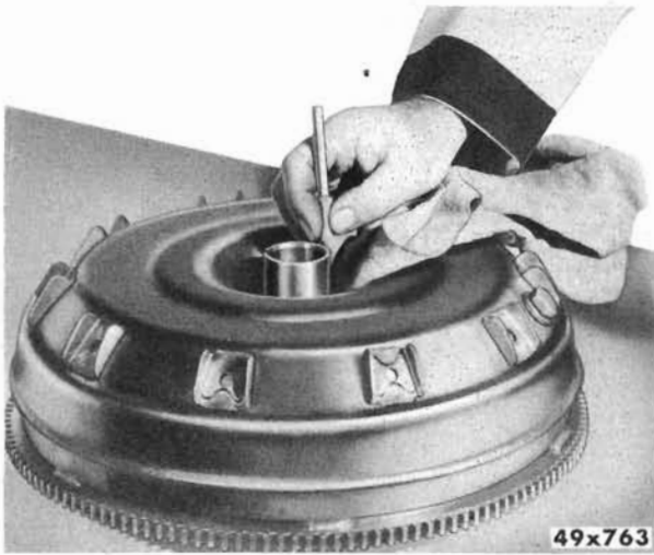
Figure 64—Cleaning Runner Hub Sealing Surface
