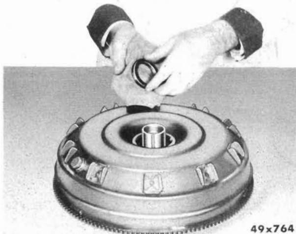
Figure 65—Cleaning Contact Surfaces of Seal Ring
