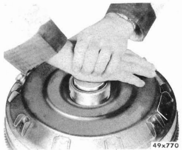
Figure 71—Installing Snap Ring
