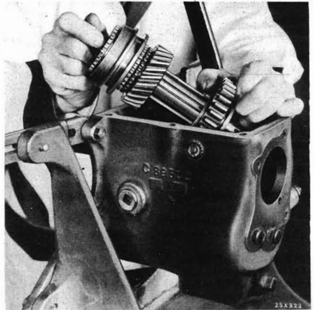
Figure 103—Removing Mainshaft Assembly (3-Speed)
