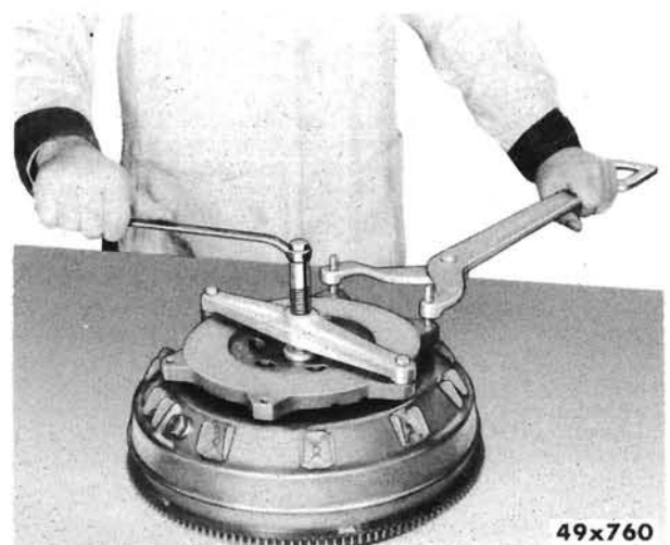
Figure 58—Removing Clutch Driving Plate
