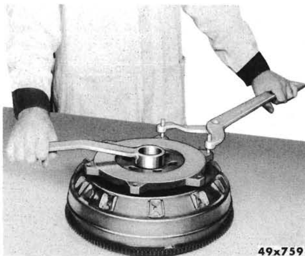
Figure 57—Removing Clutch Plate Nut
