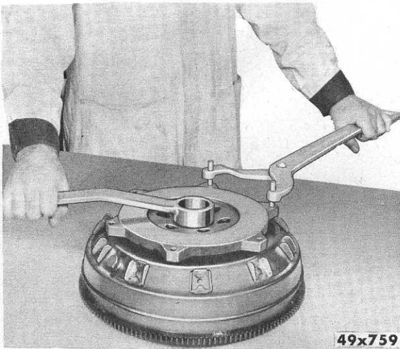
Fig. 6—Removing Clutch Drive Plate Retainer Nut
