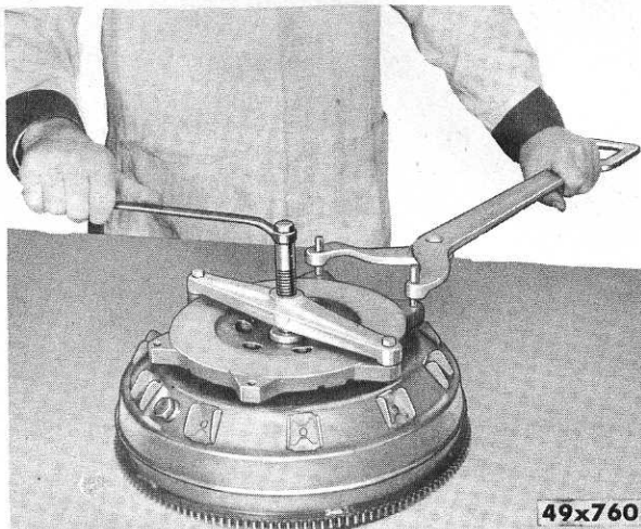
Fig. 7—Removing Clutch Drive Plate
