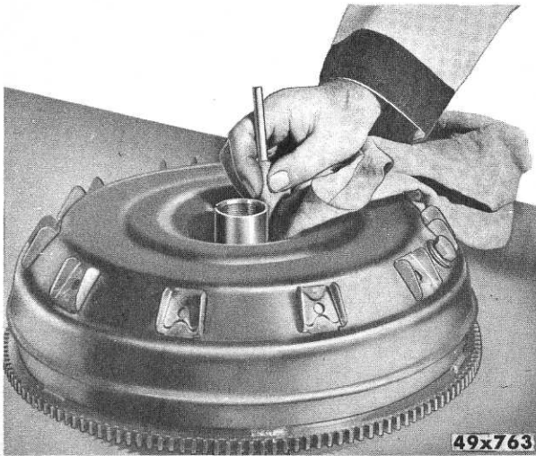
Fig. 11—Cleaning Runner Hub Sealing Surface
