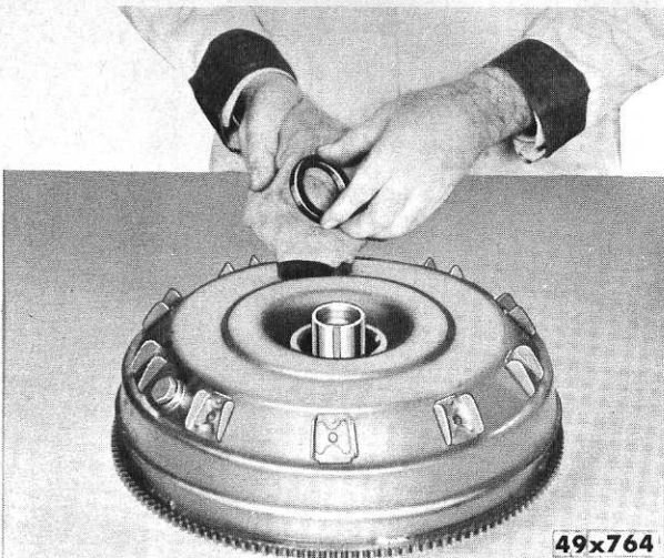
Fig. 12—Cleaning Contact Surfaces of Seal Ring
