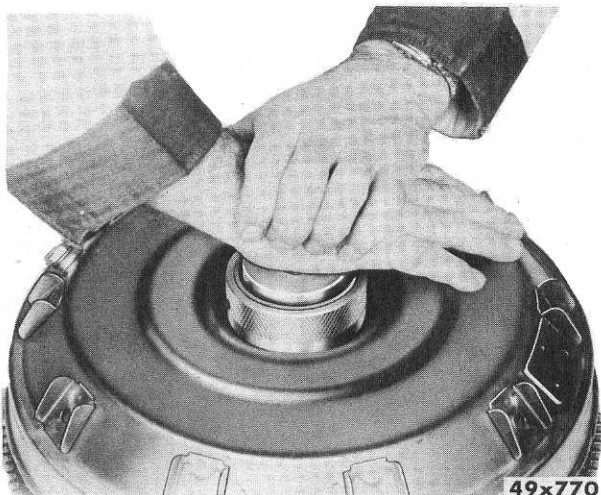
Fig. 18—Installing Snap Ring
