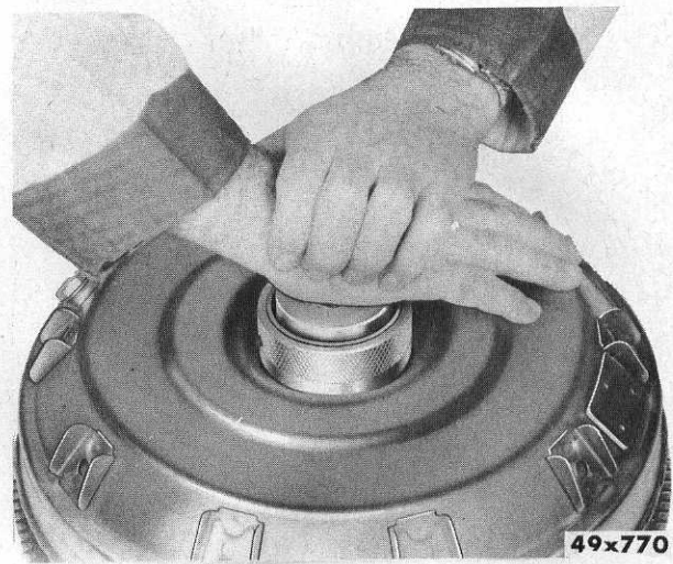
Fig. 26—Installing Snap Ring (Tool C-884)
