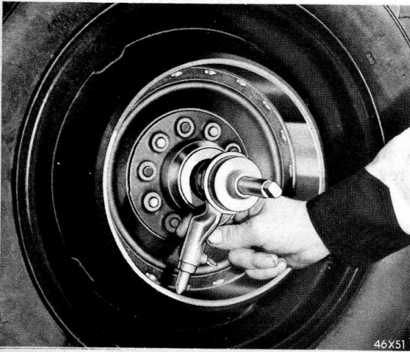
Fig. 28—Checking Brake Drum Diameter, Tool MT-34-B
