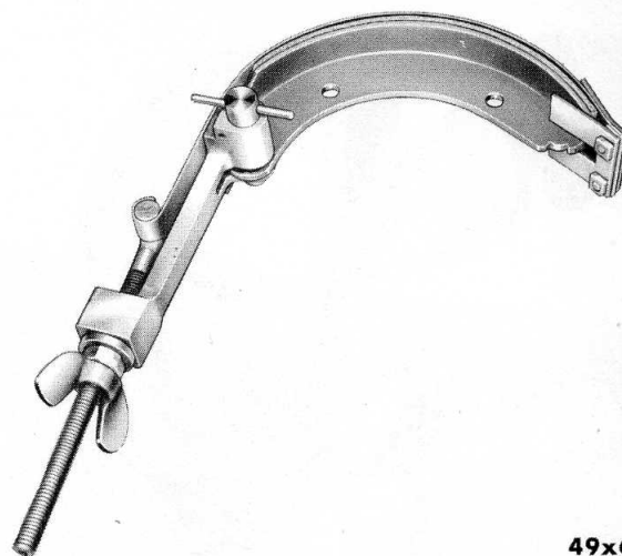
Fig. 17—Tightening Wing Nut to Compress Pressure Spring
