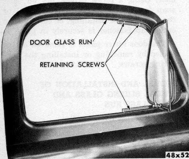
Fig. 4—Location of Ventilator Window Retaining Screws
