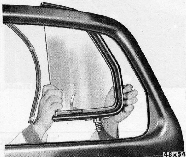
Fig. 6—Removing Ventilator Assembly
