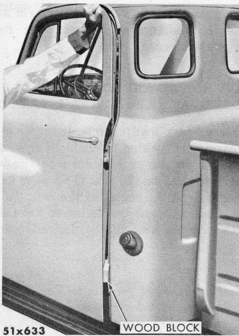
Fig. 11—Correcting Warped Door by Use of Wood Block
