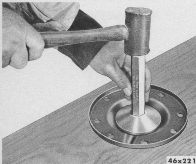
Fig. 55—Installing Pinion Oil Seal in Retainer, Tool DD-951 or DD-954
