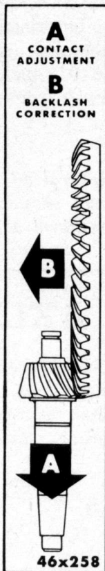
Fig. 91—Incorrect Low Narrow Tooth Contact
