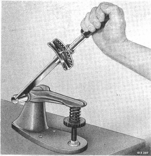
Fig. 42—Testing Valve Springs
